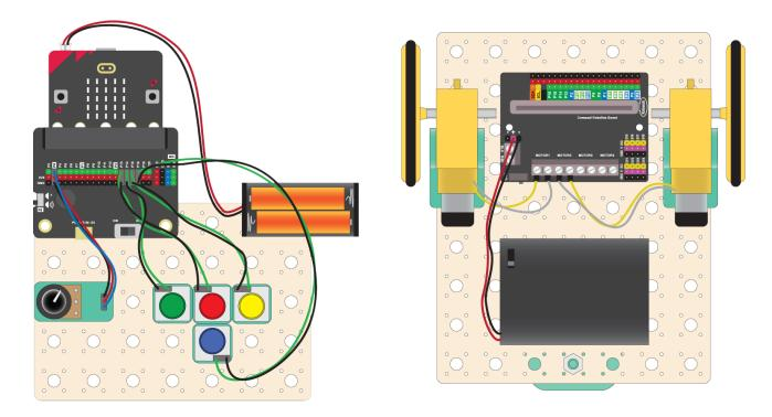
For the speed control you add a potentiometer to the remote control. This is an analogue input device. By turning the knob, you can get different values from 0 to 100 which can be used to set the speed. When we read the value from the potentiometer on the controller, we need to send the value across to the robot, so it can adjust its speed
